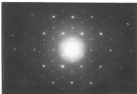
Figure 4 Electron diffraction patterns of the acicular platelets in Fig. 3a. The electron beam was incident normal to the c -axis.
